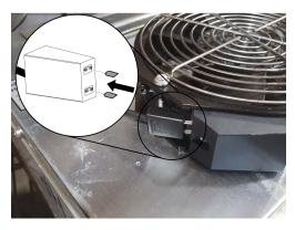
Inspect the spindle fan cable connection. Make sure both spade connectors are properly going into the female connector.
