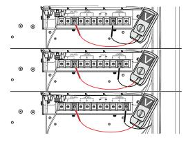
**Corrective Action:** Disconnect the motor cables at the vector drive. Push **[POWER ON]**. Push **[RESET]** to clear any alarms. Use a multimeter to measure the DC voltage across the following terminals on the vector drive (see the illustration):
